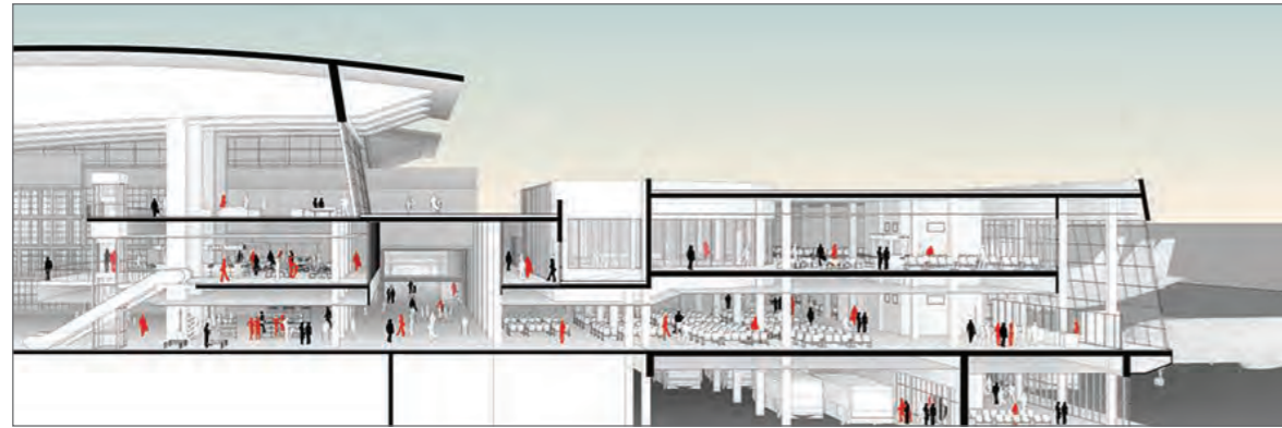
Image 3. Building layout planning: Alternative options were developed and iteratively discussed with the client, with BIM models used as the basis for visualization and data extraction. This approach helped us quickly convey the building concept and flows, supported by live key data such as gross floor area, net floor area (i.e. floor space per user) and processing numbers (check-in, security lines, baggage claim length/number, and passport control, for example).
